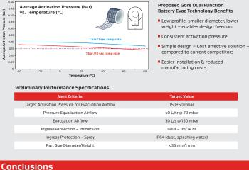
Optimal protection of battery modules from environmental perils such as moisture & particulate ingress and damage from pressure differentials can be achieved through protective venting strategies. Gore offers a combination of commercial industry-leading protective venting products, developmental protective technology and expertise in venting and conditional modeling to ensure our customers have optimal protection for battery and electronic modules.
