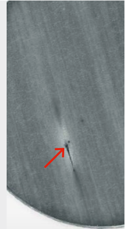
Figure 1: Not acceptable — pin hole in vent
