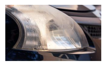
With the increase in EV production, we are seeing a lot of inquiries on moisture management for inverters, control units, sensors, and electric motors. By leveraging our experience in condensation reduction for automotive lighting, we can identify multiple materials on the inside that are sources of moisture and propose potential venting solutions. Similarly, for thermal management, we are drawing from our portable electronics portfolio, constantly trying to
