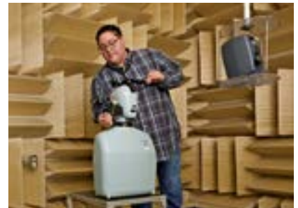
Acoustic testing inside Gore's anechoic chamber
