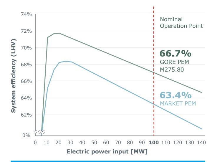
Highest system efficiency is enabled with Gore PEM M275.80 – not only at nominal power but also in part load.
