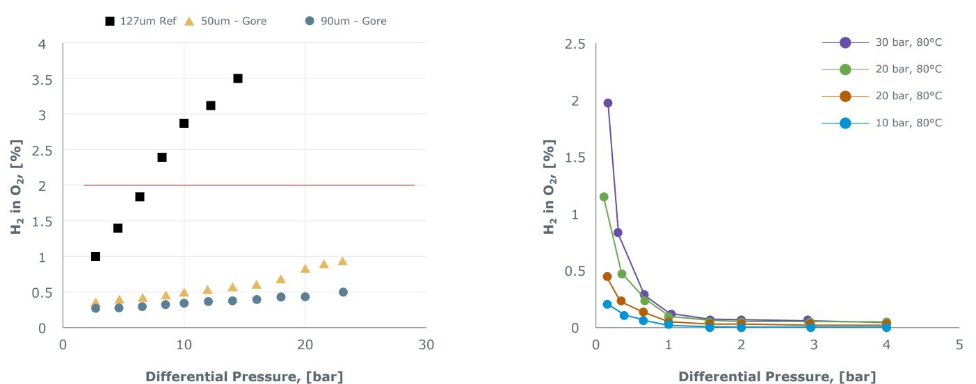
Gore RC technology shows effectiveness at mitigating  $H_2$  in  $O_2$  safety concerns. Enables high system utilization and efficiency through a wide operating range.
