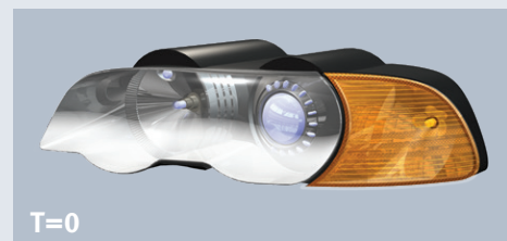
Lamp A – Final clearing time: 130 minutes
