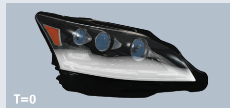
Lamp B – Final clearing time: 20 minutes
