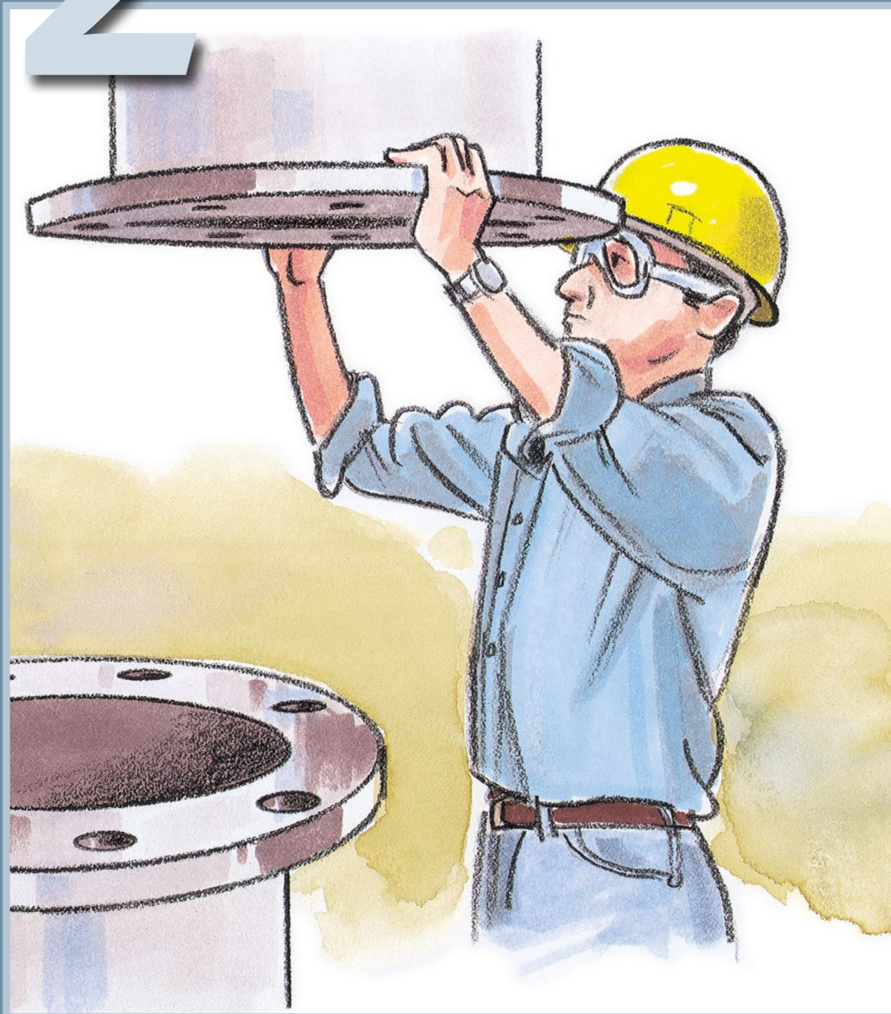
5 Install and tighten bolts as per the torque values recommended by the gasket manufacturer
