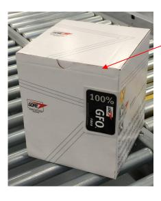
Sticker not used as a seal of the interface of box front panel with box top panel
