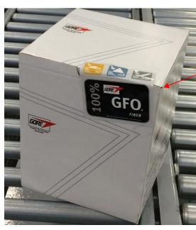
Sticker improperly aligned with the box edges
