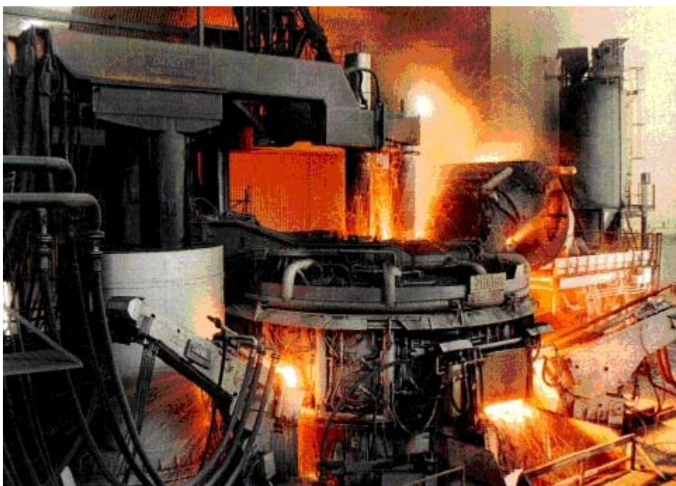
The 135-mt twin-electrode DC furnace built for Hylsa in Monterrey by Danieli.
